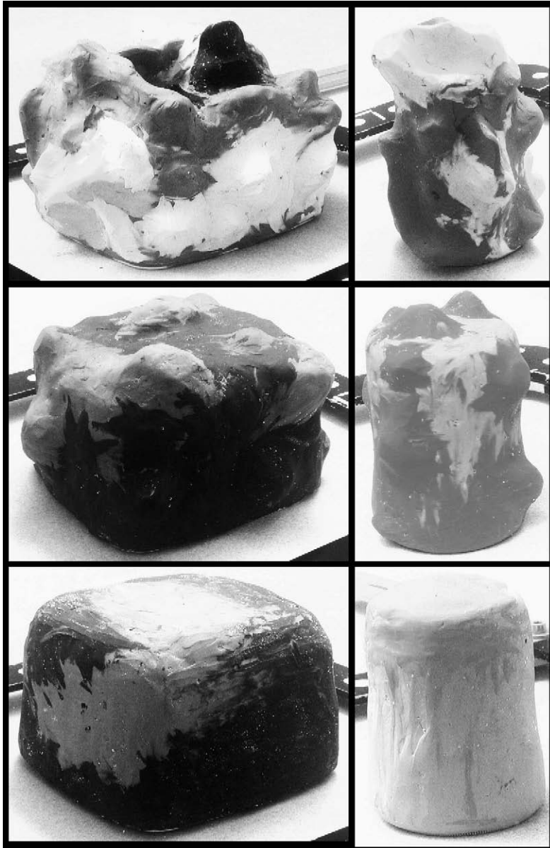
Fig. 5. Models used to evaluate the volume measuring technique. The large (left) and small (right) complexity models are the top images, moderate large (left) and small (right) complexity models are the middle images, and the large (left) and small (right) simple complexity models are the bottom images.
