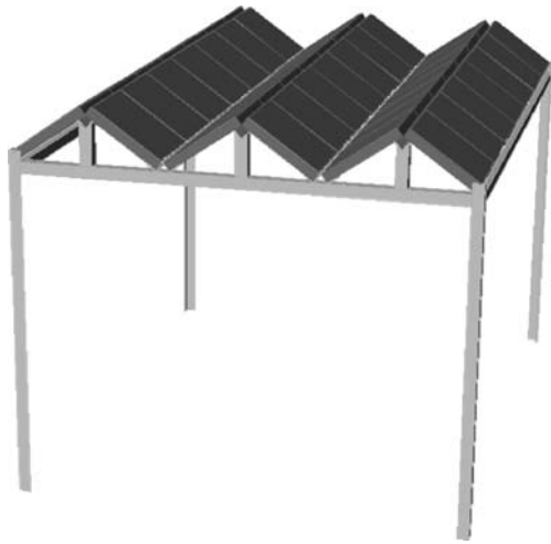
Fig. 2 Platform that was placed at the study site containing 42 tiles, sponges were attached on every tile. Size platform: 2.5-m×1.6-m×1.2-m
